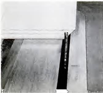
DELUXE, LOCKED-MITER CORNER , shown above, uses an L-shaped spline for accurate alignment and maximum strength. A dado head is useful but not necessary for cutting the \frac{1}{4} "-wide grooves that take the splines. If you use a regular blade, run off \frac{1}{2} "-deep kerfs to form the outer edges of each groove. In photo below, at
